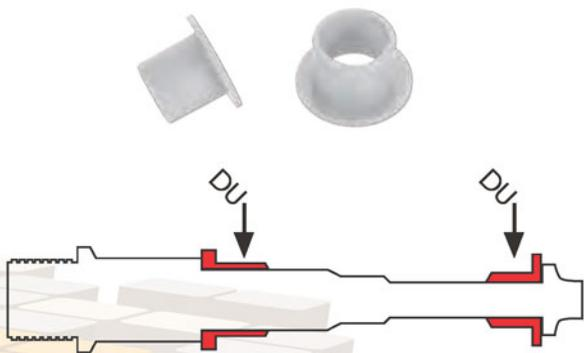
Patent design for 2 DU bushing unique construction
